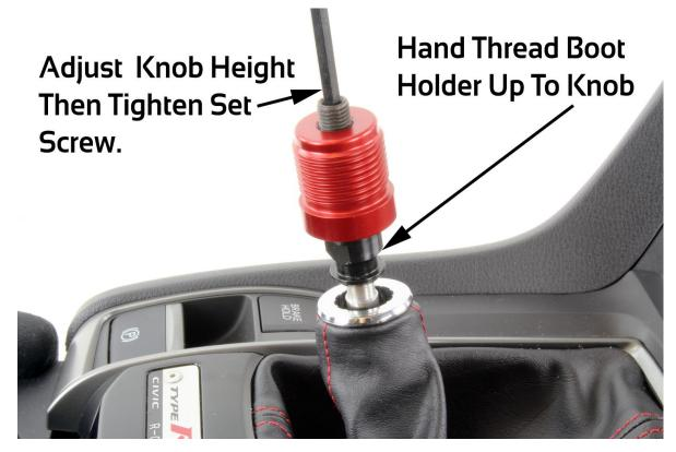
4. Install shift knob to shifter and follow instructions for height and rotation adjustment.
