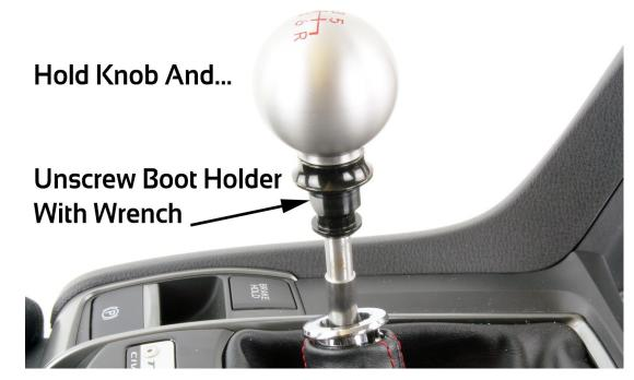
3. Remove shift knob making sure to leave lower boot holder/nut installed. Screw lower boot holder/nut down until it stops.
